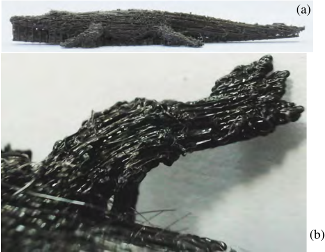
Figure 19: Manufactured object for a model of a crocodile (the support structure was not removed), created using the method presented in Section 4.2. In (a), the whole object is shown. (b) gives a more detailed view of the back right leg. See also Figure 6.
