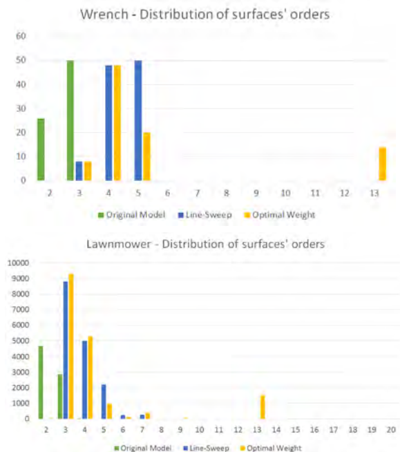
Figure 20: The distribution of orders in the input and output surfaces for the Wrench model in Figure 11 (top) and for the Lawnmower in Figure 16 (bottom). Note we count instances, having two instances of orders per surface, being a bivariate function.
