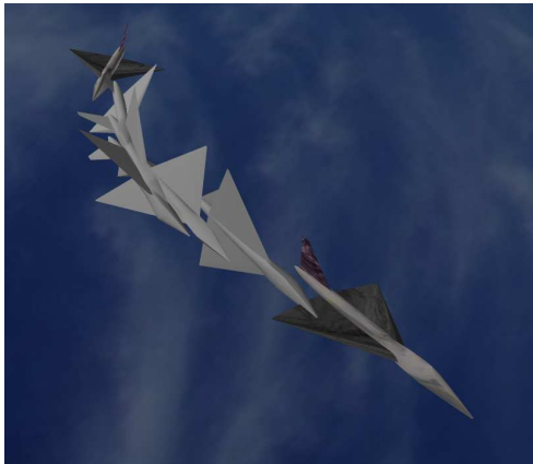
Figure 9. (a) Flying motion of a plane and (b) the corresponding sweep envelope surface, the result of solving Equation (4).
