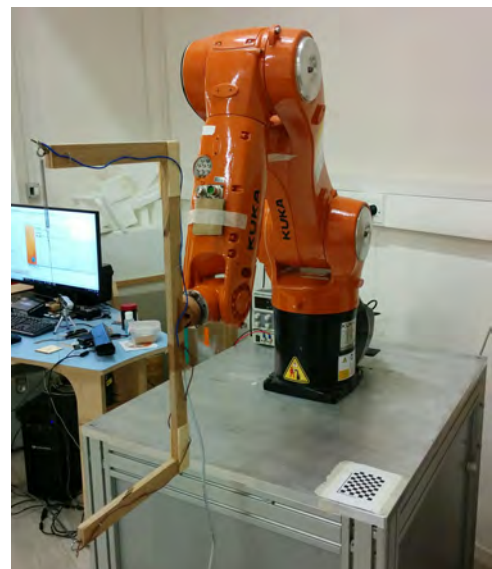
Figure 1: A hot-wire cutting configuration based on a 6-DoF robot arm.
