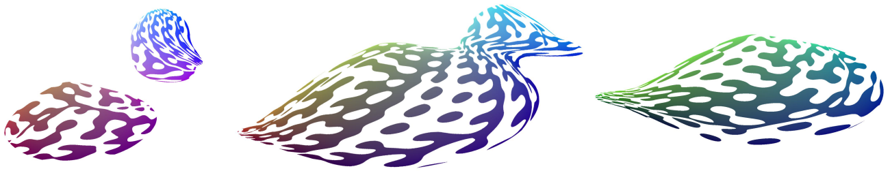
Figure 6: The top row shows a marching cubes' polygonal approximation of a heterogeneous duck model tiled with Gyroid tiles. One tile is highlighted in cyan. Bottom row shows the same model, 3D printed, from similar views.
