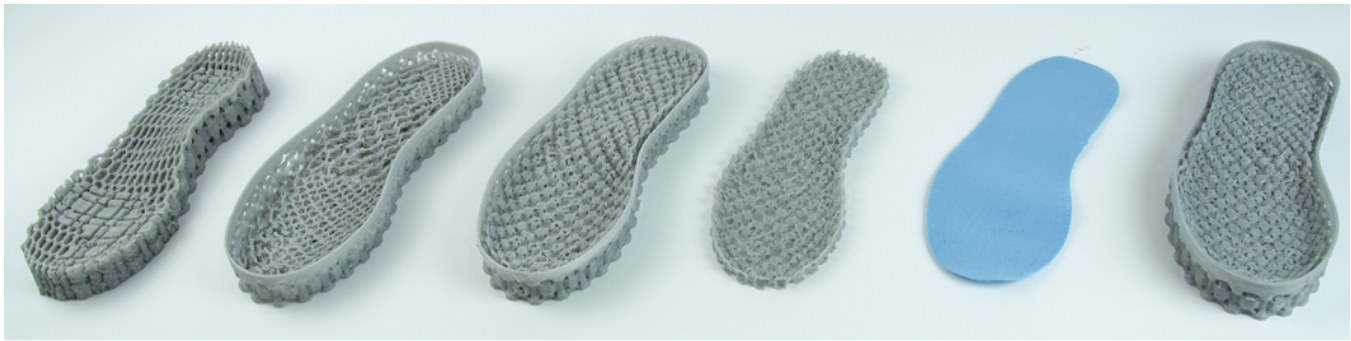
Figure 11: Sole tests, including insole, midsole and outsole tests 3D printed (FDM) in Filaflex.
