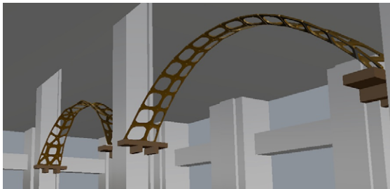
Fig. 13. Two designs for chocolate arches that span the 3.75 m between structural columns, resting on temporary platforms.
