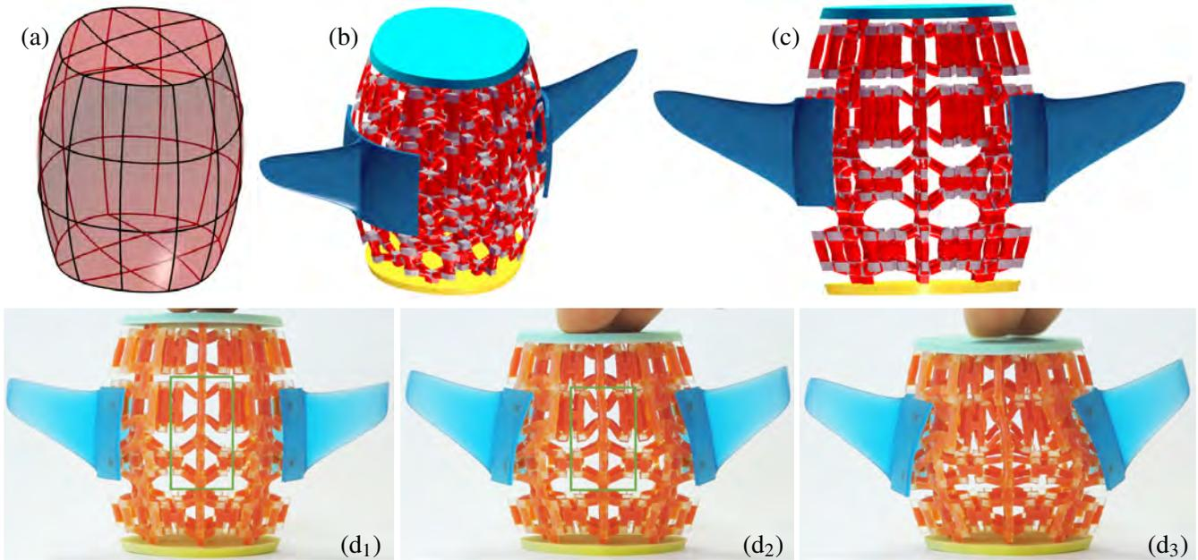
**Figure 7:** An Auxetic based compliant microstructure mechanism, in a 3D barrel shape (a). Tiles from the family of tiles in Figure 6 are functionally composed into this barrel macro-shape trivariate  $\mathcal{M}$  that is shown in (a). The full computer model with a base, top, and side wings is shown in (c) and (d). Then  $(f_1)$  to  $(f_3)$  are snapshots from a movie (<https://youtu.be/NKck4N7TKQI>) captured of this 3D printed model undergoing vertical pressure.
