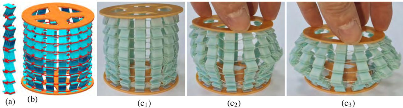
**Figure 5:** A radial shear compliant microstructure mechanism. The column of eight different shear tiles, in (a), is placed around a cylinder (16 times) to yield (b). (c<sub>1</sub>) to (c<sub>3</sub>) show the model undergoing vertical pressure, and are from the short video ([https://youtu.be/XyXgDm61\\_Lc](https://youtu.be/XyXgDm61_Lc)). Note This variation of shear tile also employs small joints to its two immediate adjacent tiles, for stability under pressure.
