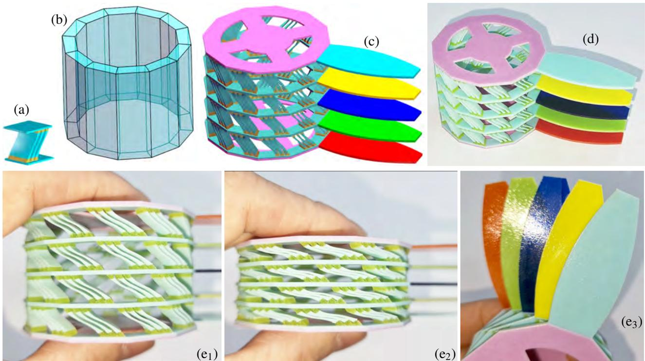
**Figure 4:** A rounded twisting compliant microstructure mechanism. The shear tile in (a) is populating (many times) the trivariate macro-model  $M$  in (b), via functional composition, and the final model is shown in (c). In (d), the 3D printed model is presented, and (e<sub>1</sub>) to (e<sub>3</sub>) are snapshots from the short video (<https://youtu.be/c3QUUFxBOyI>), of the mechanism undergoing vertical pressure.
