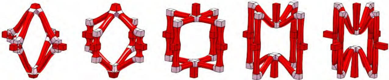
**Figure 6:** Several samples of different parametric Auxetic tiles that are heterogeneous, with rigid (in red) and flexible (in light-grey) materials.
