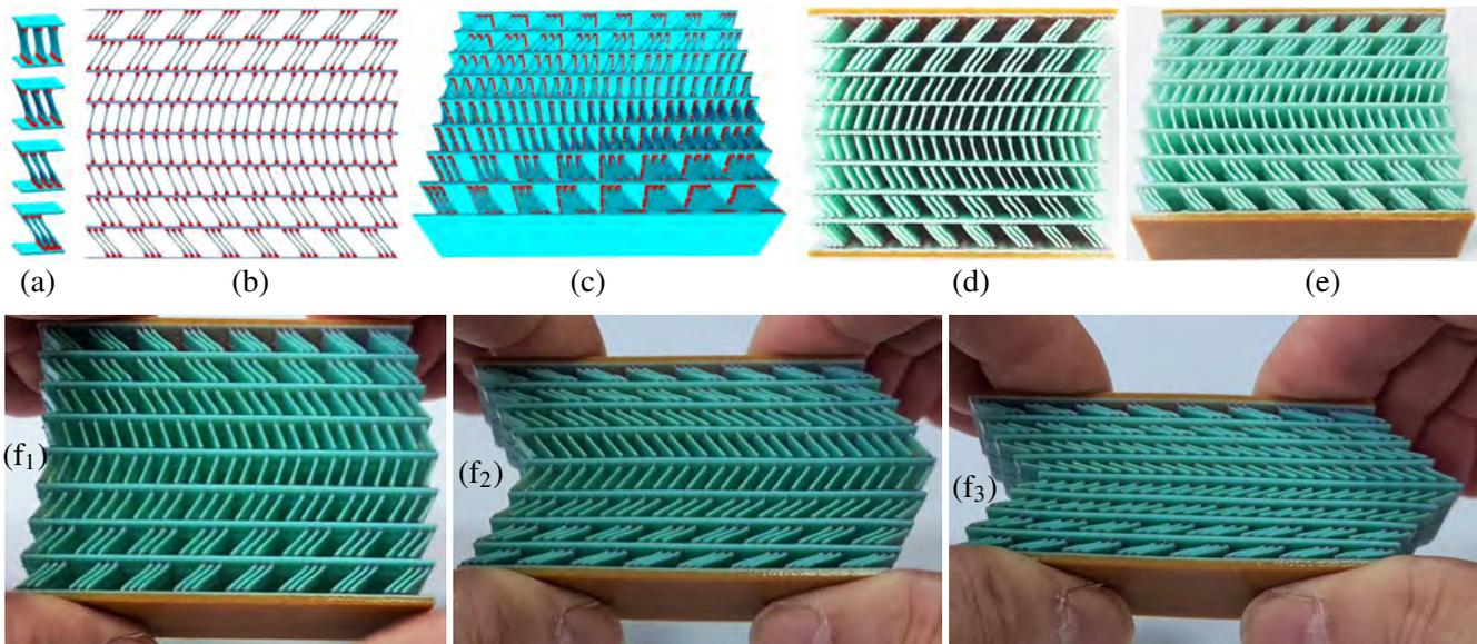
**Figure 3:** A linear shear compliant microstructure mechanism. In (a), the different shear tiles, that are employed in this model, are presented. (b) and (c) present the 3D final result,  $M(\mathcal{G})$ , as a computer model whereas (d) and (e) show the 3D printed counterpart. Finally, (f<sub>1</sub>) to (f<sub>3</sub>) are three snapshots captured from a movie (<https://youtu.be/gJ4XecdAB4Q>) of this 3D printed model undergoing vertical pressure.
