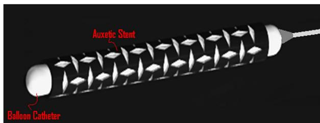
**Fig. 16** A schematic showing an Auxetic stent mounted on a balloon catheter
