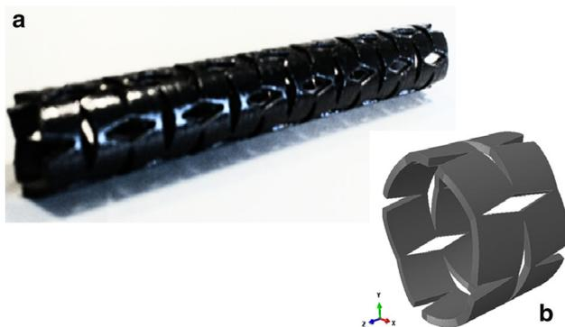
**Fig. 53** **a** Auxetic Oesophageal Stent (physical), **b** Auxetic-ring FEA model
