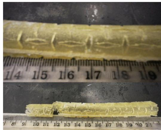
**Fig. 6** A fractured Auxetic polyurethane stent having being released from the tubular die
