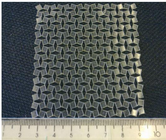
**Fig. 1** Lasercut Auxetic polyurethane film
