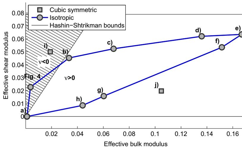
**Fig. 9.** Hashin-Shtrikman bounds and effective moduli for several topology optimized designs. The base material properties are the same as for the structure in Fig. 10, and the volume fraction of the blueprint design is constrained to 33.8% (corresponding to the design in Fig. 10). Unit cells corresponding to the points are shown in Fig. 10.
