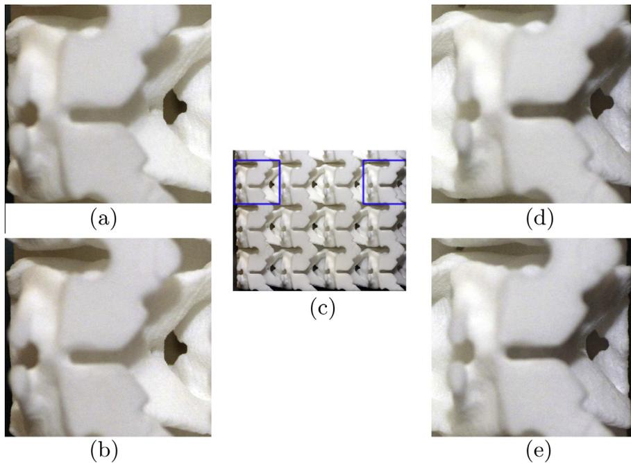
**Fig. 8.** Visualization of the structure deformations. (a) Undeformed unit cell on left side, (b) deformed version. (d) Undeformed unit cell on right side, (e) deformed version. (c) Three bottom rows of the sample. The blue selections indicate the positions of the close ups. The negative Poisson's ratio behavior is illustrated by how both sides contract (the black edge area becomes larger).
