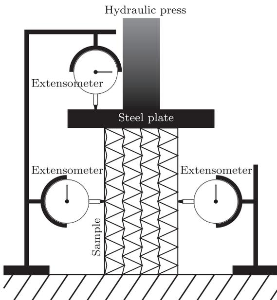
**Fig. 5.** Experimental setup for measurements of Poisson's ratio.
