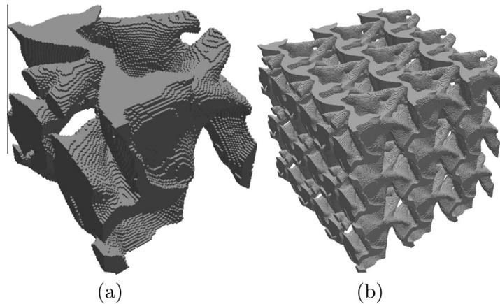
**Fig. 4.** 3D isotropic microstructure with Poisson's ratio  $-0.51$ .  $a = 0.125\%$  is used for the stiffness constraint on the eroded design, while the isotropy constraint parameter  $\epsilon$  is set to  $10^{-5}$  for all three designs. The solid volume fraction of the dilated design is constrained to 40%. The initial guess is a random distribution of densities. (a) One unit cell. (b)  $3 \times 3 \times 3$  unit cells.
