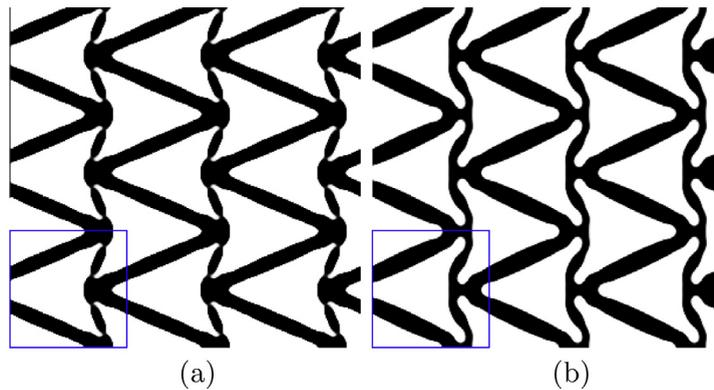
**Fig. 2.** Negative Poisson's ratio structures obtained with (a) a projection, and (b) robust formulation. Parameters are the same as for the designs in Fig. 1, except for the volume constraint in the robust formulation, which is applied on the dilated design and is set 15 percent higher. The design in Fig. 1(a) is used as the initial guess.
