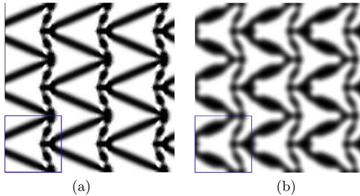
**Fig. 1.** Minimum Poisson's ratio design obtained with standard filtering. In both cases a linearly decaying filter with a radius of 1/10 of the unit cell length was used. Other parameters are:  $a = 0.2\%$ ,  $\epsilon = 10^{-5}$ ,  $N = 10000$ , and  $V = 35\%$ . (a) Sensitivity filter started from a random distribution of densities. (b) Density filter started from the design in (a). The box in the corner encloses one unit cell.
